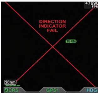
Figure 4-86 Direction Indicator Fail
