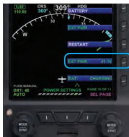
Figure 6-3 External Power Voltage Status
