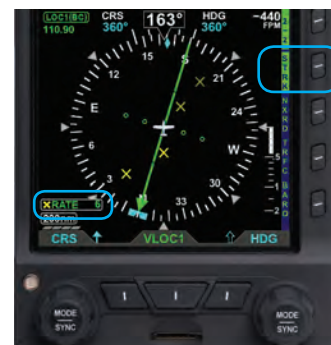
Figure 3-35 Lightning Overlay On Displaying WX-500 Strike Data
