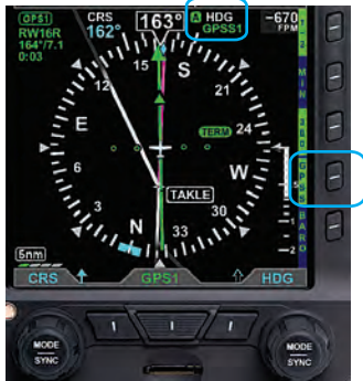
Figure 6-9 Operating in GPSS Mode
