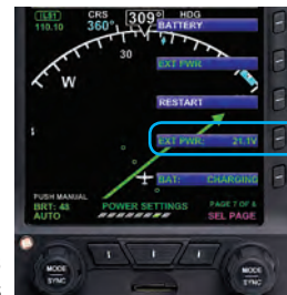
Figure 6-3 External Power Voltage Status
