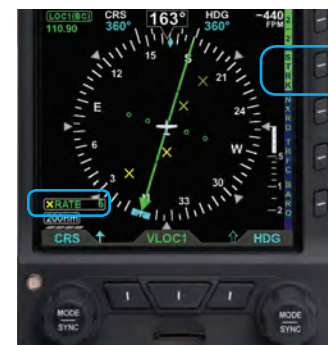
Figure 3-18 Lightning Overlay On Displaying WX-500 Strike Data
