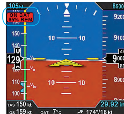
Figure 6-2 Battery Charge Remaining
