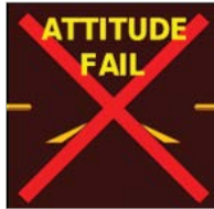
Figure 1-6 Attitude Failure Indication
